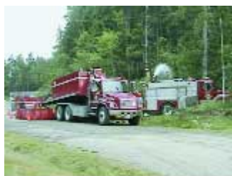
During the test the department achieved a water flow of 200-lgpm, uninterrupted for a total of two hours.
