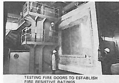
TESTING FIRE DOORS TO ESTABLISH FIRE RESISTIVE RATINGS
